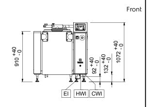
CWII Cold Water inlet 1 (cleaning) Electrical inlet (power) HWI Hot water inlet
